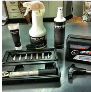
From top left to bottom right: Carbon Grease Compound, Carbon cleaner, Carbon Polish Adjustable Value Torque wrench, And a Fixed Value Torque wrench.
